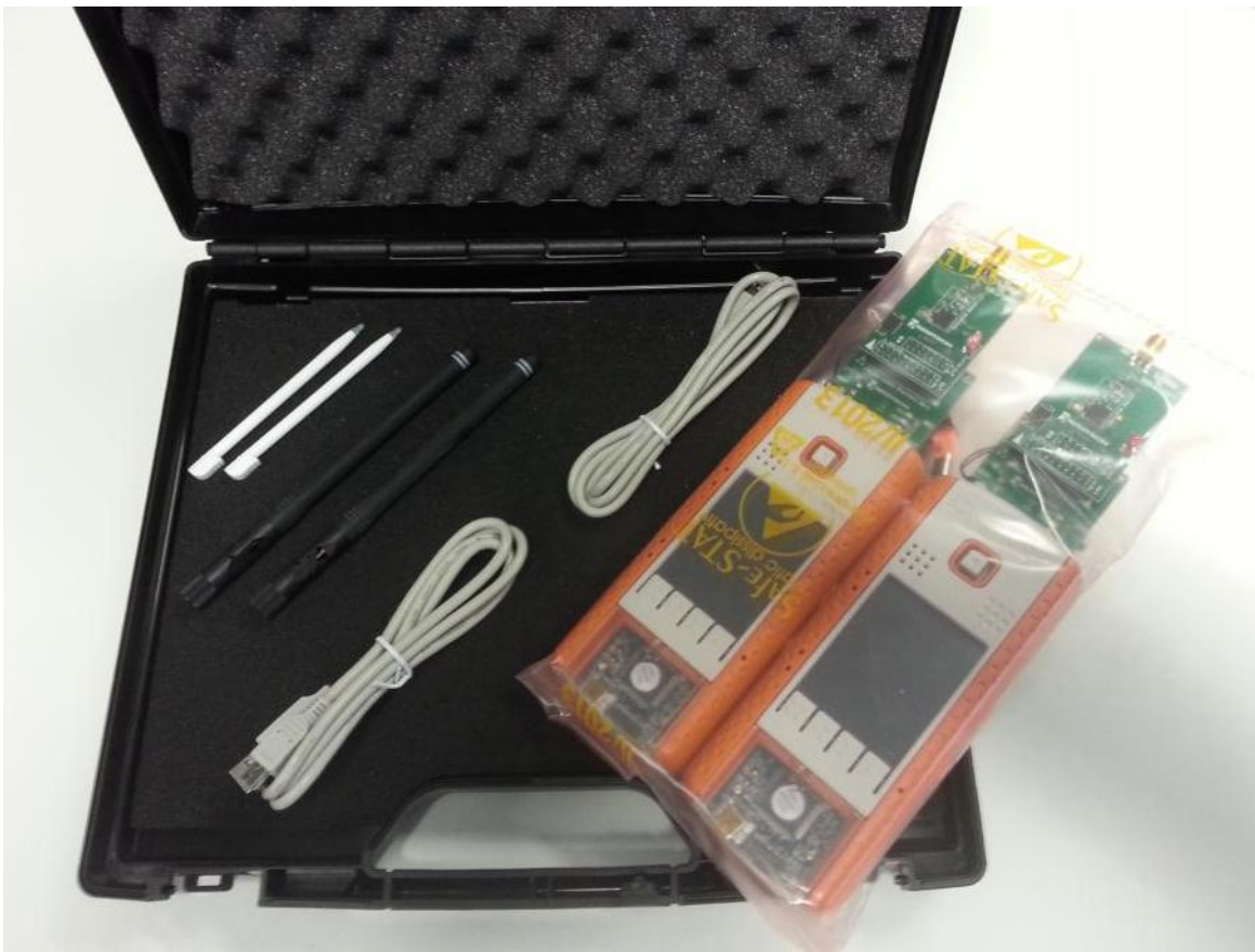
Figure 1: SX1272 Development Kit (SX1272DVK1BAS - 868MHz version)
