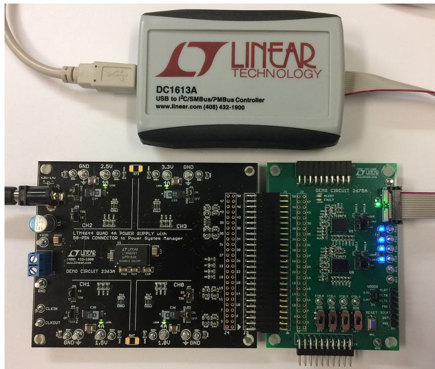
Figure 3. Connecting DC2363A/DC2675A Boards and the DC1613 USB to I 2 C/SMBus/PMBus Controller
