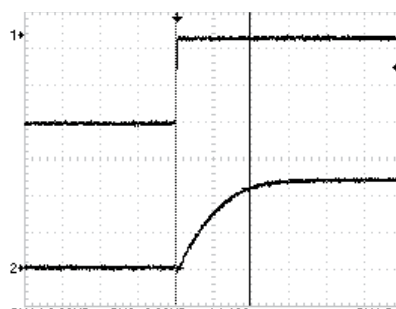
Typical Start-Up Wave Form
