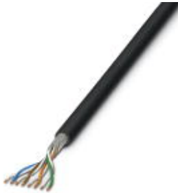
CAT5e-SF/UTP cable, 4 x 2 x 26 AWG, stranded (7-wire), shielded, outer sheath: PVC, outside diameter 6.4 mm, cable ring 100 m
