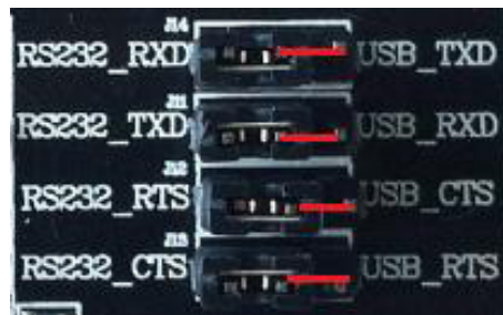
Figure 5: USB to serial jumper connect
