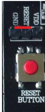
Figure 9: Jumper setting for low effective RESET
