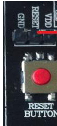
Figure 8: Jumper setting for high effective RESET
