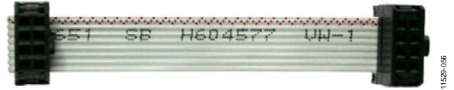
Figure 55. Parallel Cable to Connect Two Evaluation Boards
