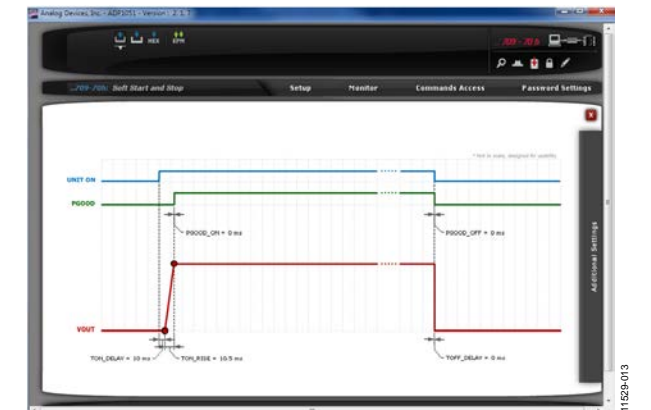
Figure 13. Soft Start and Stop Settings Window
