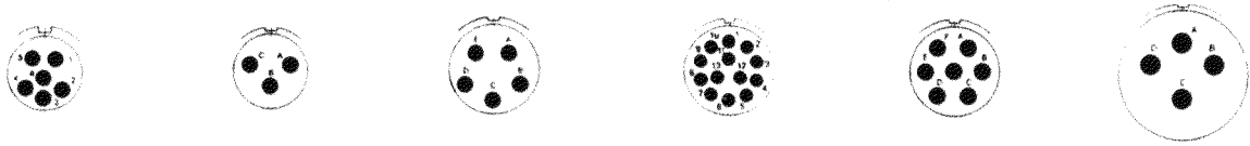
09-35 6 SIZE 22D CONTACTS 09-98 3 SIZE 20 CONTACTS 11-05 5 SIZE 20 CONTACTS 11-35 13 SIZE 22D CONTACTS 11-99 7 SIZE 20 CONTACTS 13-04 4 SIZE 16 CONTACTS
