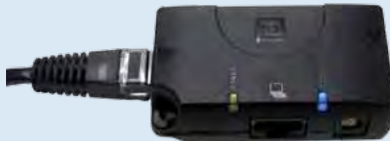
Power LED and IEEE802.3at LED illuminate when connected to compliant IEEE802.3at load.
