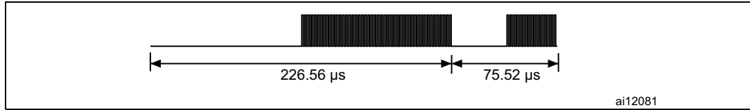
Figure 38. Start of frame, low data rate, one subcarrier, fast commands
