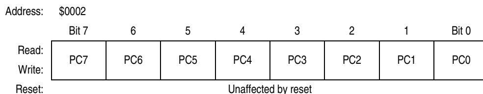
Figure 7-13. Port C Data Register (PORTC)
