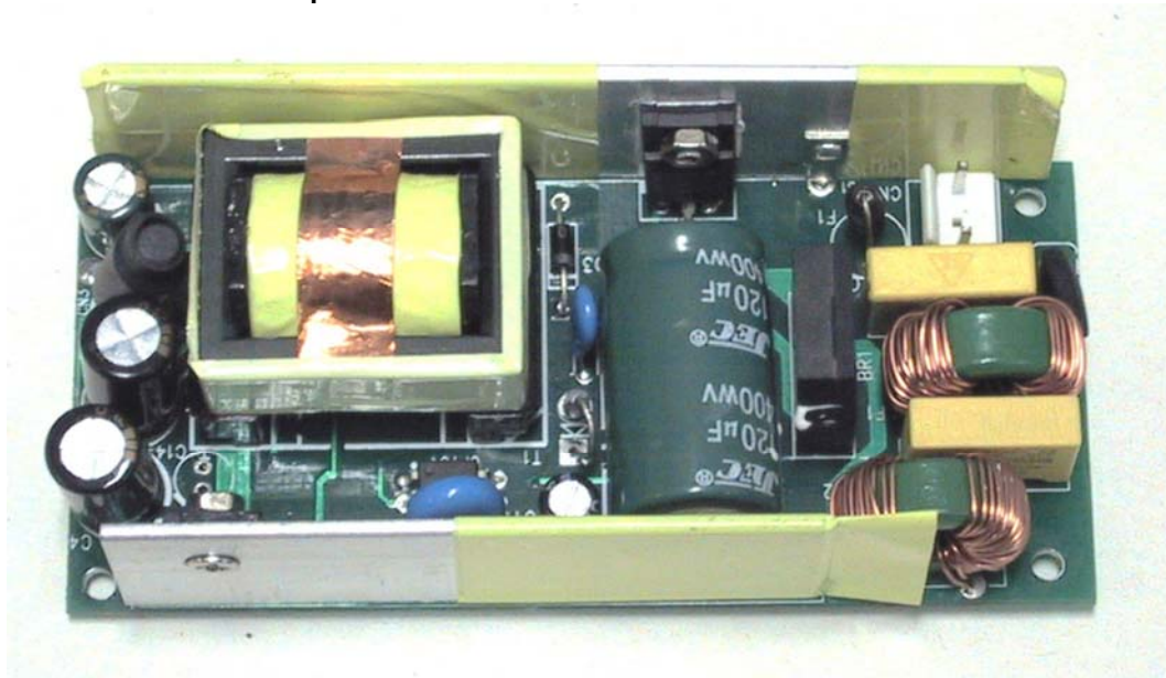
Figure 1: EVL6566B-65W Adapter demo-board
