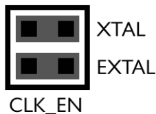
Figure 6-23: External Crystal Circuitry Enable (J22)
