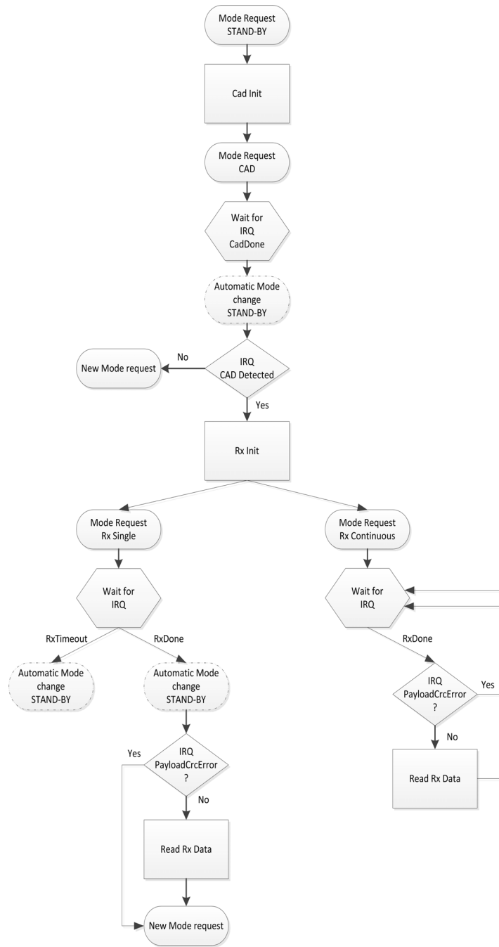
Figure 12. LoRa™ CAD flow
