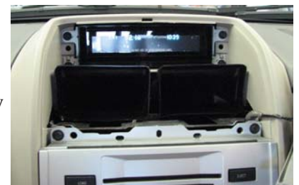
Air Vent Assembly Removed
