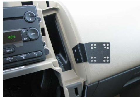
InDash Installed, Mounting Location - Edge
