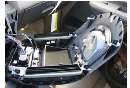
Radio Climate Control, Air Vent, Bezel Removed
