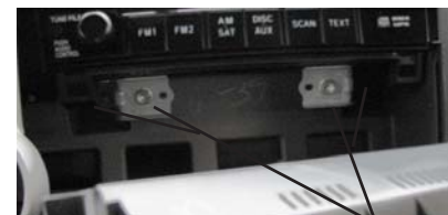
(4) Radio bolts Location
