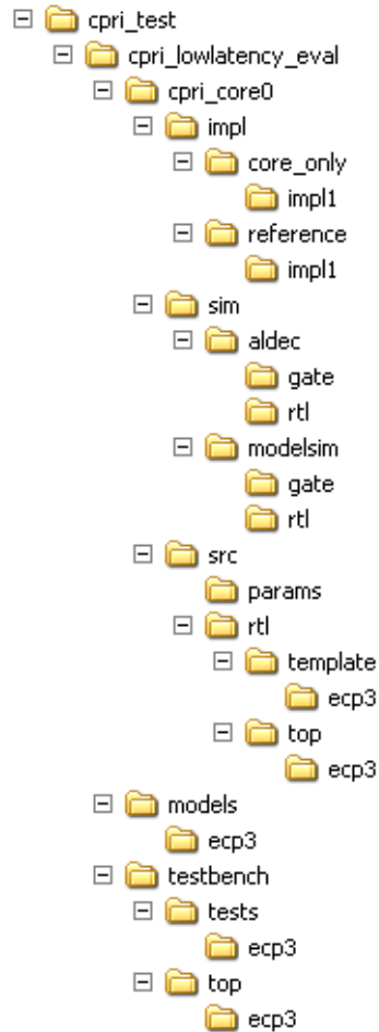
Figure 4-5. LatticeECP3 CPRI IP Core Directory Structure
