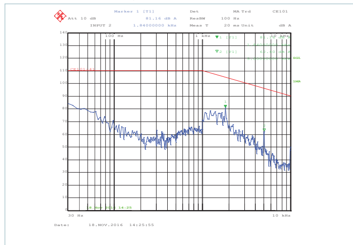
Figure 7 — Peak scan for the BLACK lead with C_{IN} = 100\mu F , C_{OUT} = 2000\mu F , 100% load
