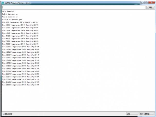
Arduino SHT20 Serial port Result
