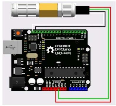
Arduino SHT20 Temperature & Humidity Sensor Connection
