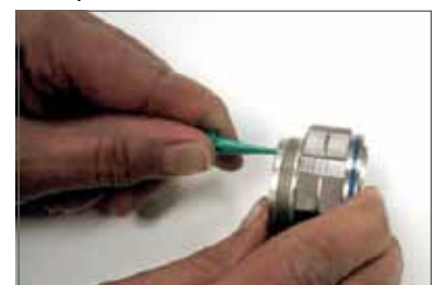
Plastic tool with contact in proper position.
