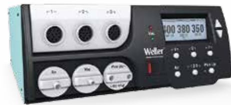
WXR3 NEW Rework power unit 273 x 235 x 102 mm (LxWxH) (10.75 x 9.25 x 4.02 inch) 6.7 kg Order No. WXR3
