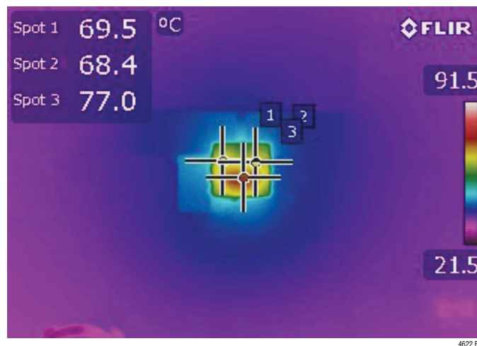
Figure 22. Thermal Picture, 12V Input, 3.3V and 5V Output, 2.5A DC Each Output with No Air Flow and No Heat Sink
