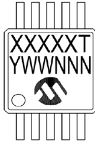
10-Lead MSOP (3x3 mm)
